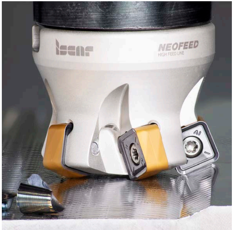
Fig 3 NEOFEED HFM tools feature the economical double-sided inserts with 8 indexable cutting edges to use on cemented carbide rationally, and a dovetail-shaped insert pocket that ensures reliable mounting to withstand heavy loads. This enables higher cutting data and increased productivity
