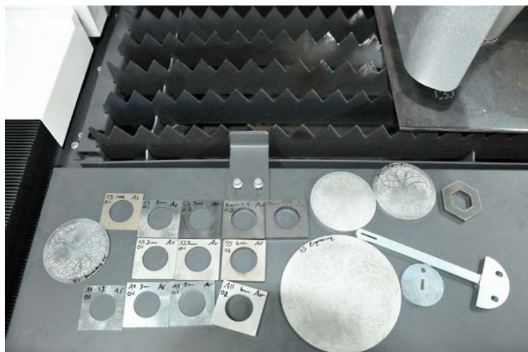
Components cut on TruSeal's new 6kW Bodor fiber CNC laser cutter – the purchase was made to control components they make from beginning to end and to also be able to speed up the time it takes to prototype and test new products. Soon to arrive is a Durma AD-S 30135 4-AXIS bending brake with 3m bending width and 135 ton bending force
