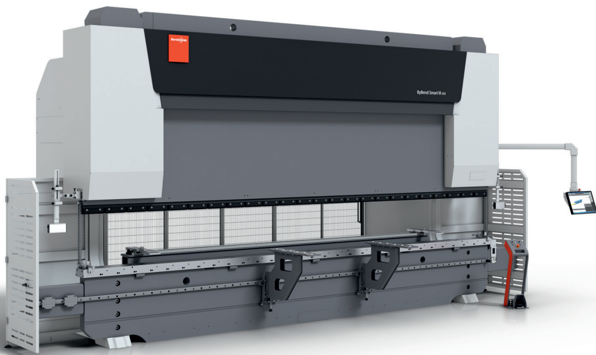
The Bystronic ByBend Smart press brakes range between 100 and 300 ton press force and a bending length between 3 100mm and 4 100mm
