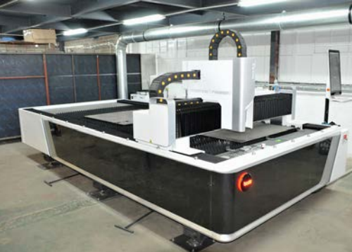
TruSeal recently installed a 6kW Bodor fiber CNC laser cutter with a 2.5m x 1.5m bed, supplied by Spectrum Machine Tools Africa
