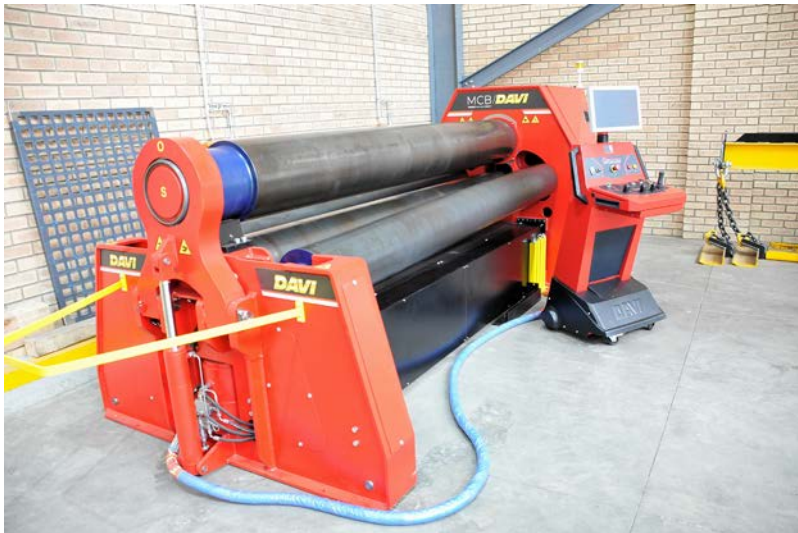
JP Engineering have added a 4-roll Davi MCB-F30 capable of rolling mild steel up to 25mm thick up to 3 040mm wide, equipped with the latest iRoll CNC console, supplied by Spectrum Machine Tools Africa
