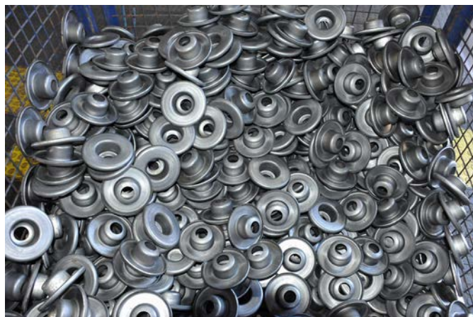
NC Idlers manufacture a range of idler components including steel and polyprop end caps, labyrinth seals, dust caps and covers, circlips, bearing housings, impact rubber discs, nylon discs and top hats. Pictured: steel end caps ready for assembly
