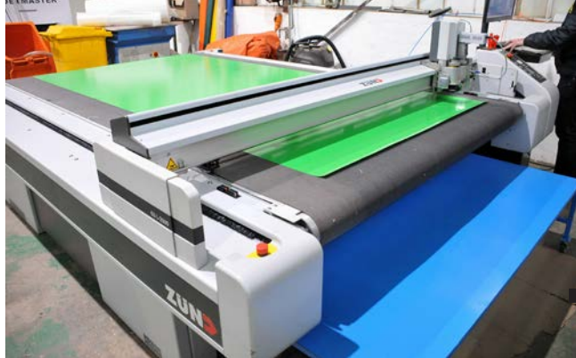
Large rolls of PVC bag material are cut with TruSeal's state-of-the-art Zünd G3 L-2500 digital CNC cutter. The Swiss-made machine features a table length of 2 500mm and a width of 1 800mm, accommodating a variety of material thicknesses
