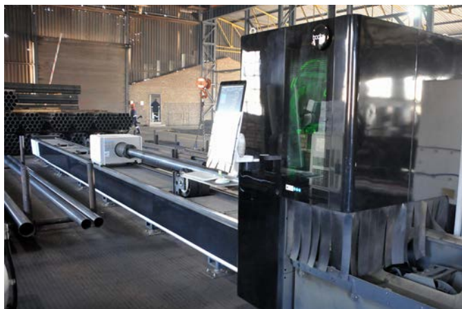
NC Idlers aims to automate their manufacturing as far as possible and the most recent machine shop upgrade was the purchase and commissioning of a Bodor 6kW K Series Tube Laser Cutter supplied by Spectrum Machine Tools Africa
