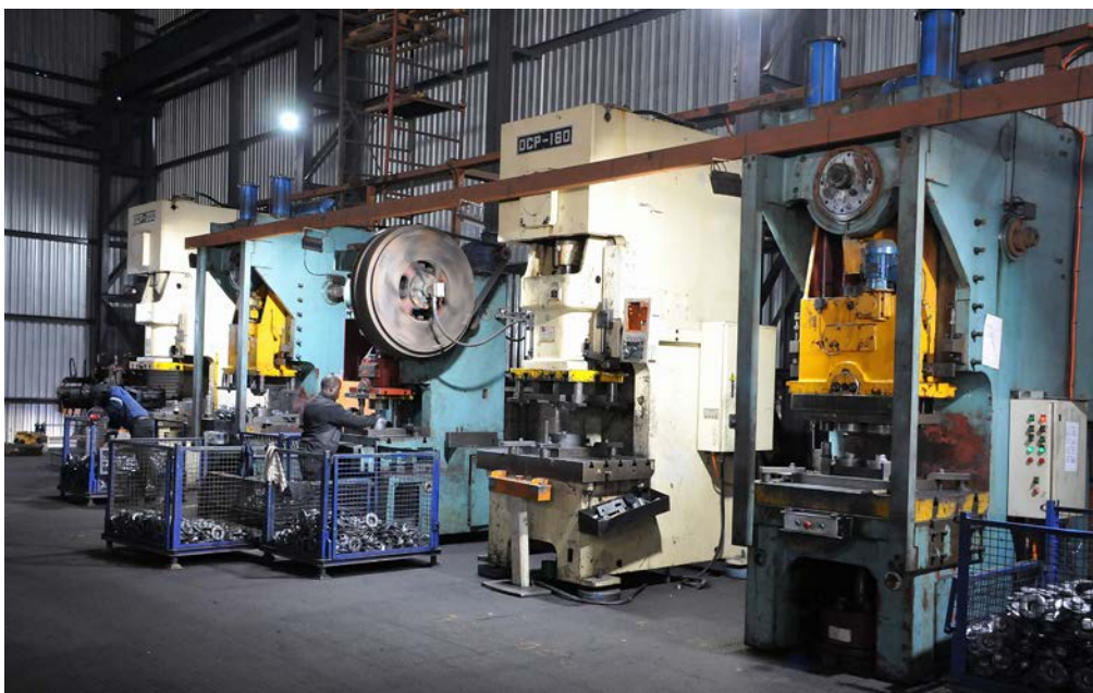
NC Idlers make use of a range of presses, both eccentric and hydraulic, to manufacture components for their idler range of products
