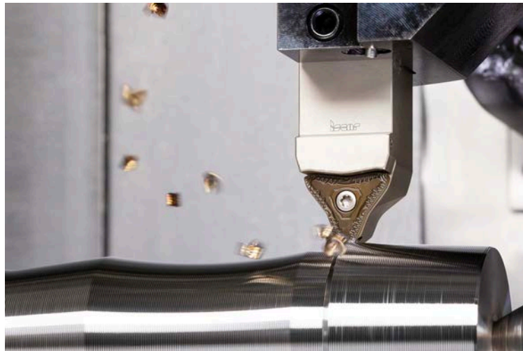
Fig 1 The advanced chipformer, which is specifically designed for high-feed turning, is a key feature of QUICK-T-LOCK indexable tool family
