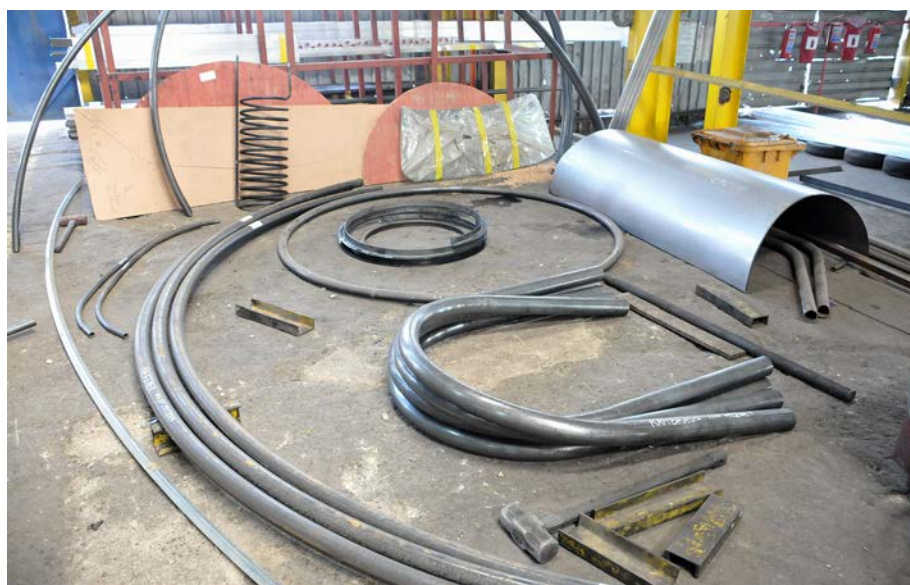
Topping Rollers can roll plates from 0.5mm down to small sizes, right up to 20mm over 3m lengths in mild steel and up to 16mm thick in stainless steel. The company's press brake is used mainly for in-house applications, however, they are able to bend 3mm mild steel plate over 2.5m
