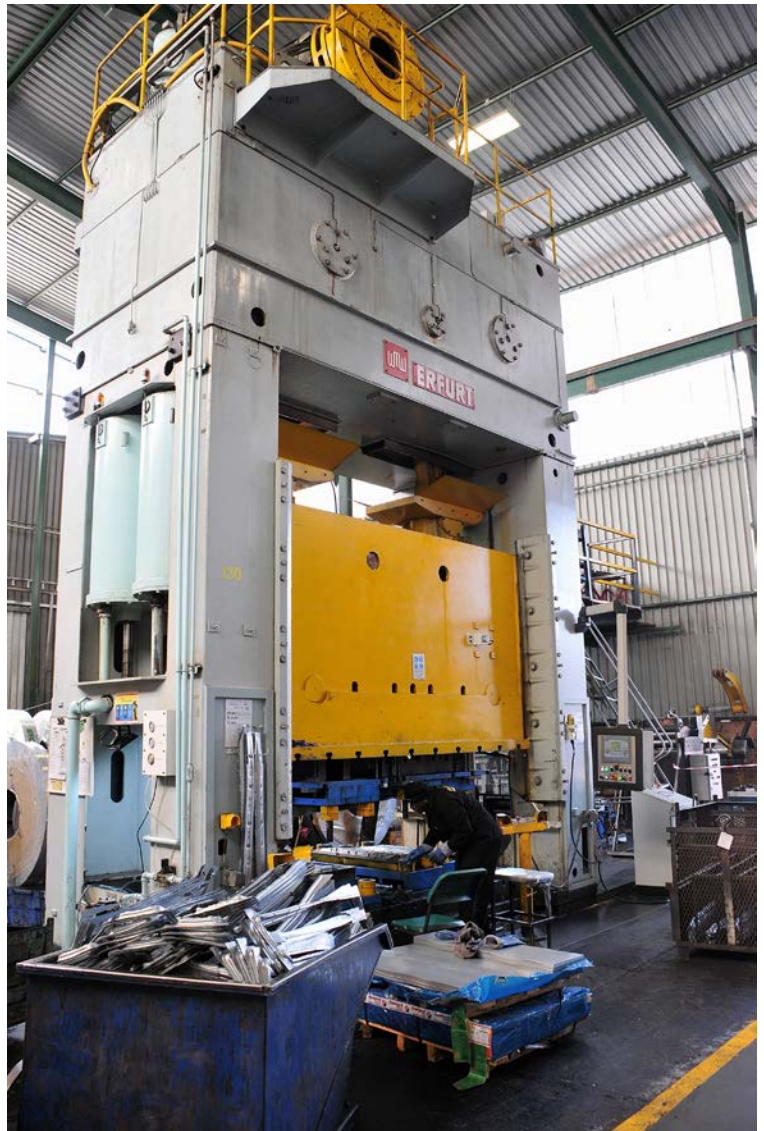
Pabar is equipped with large hydraulic presses ranging from 150 tons to 1 000 tons
