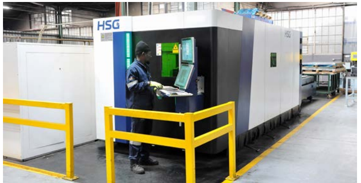
Pabar's HSG 12kW G3015X fiber laser cutter with a bed size of 3m by 1.5m, supplied by Metal Chip Machinery
