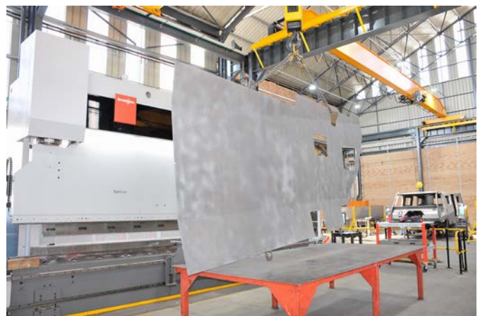
The new Bystronic Xpert 650/720 is a large machine purchased to accommodate large sheet sizes
