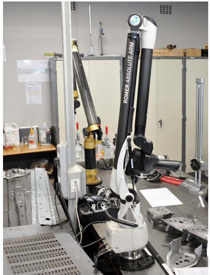
Pabar maintains certification to IATF 16949:2016 and employs advanced measuring systems such as 3D CMMs that include its Romer (now Hexagon) and Farro measuring arms, as well as digital microscopes to ensure compliance with these internationally recognised industry standards within its in-house quality and inspection office
