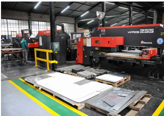
Pabar has an extensive CNC machine shop and toolroom that includes a range of CNC machines such as CNC milling machines and CNC lathes and wire EDM capabilities. Pictured are some of Pabar's Amada punching machines
