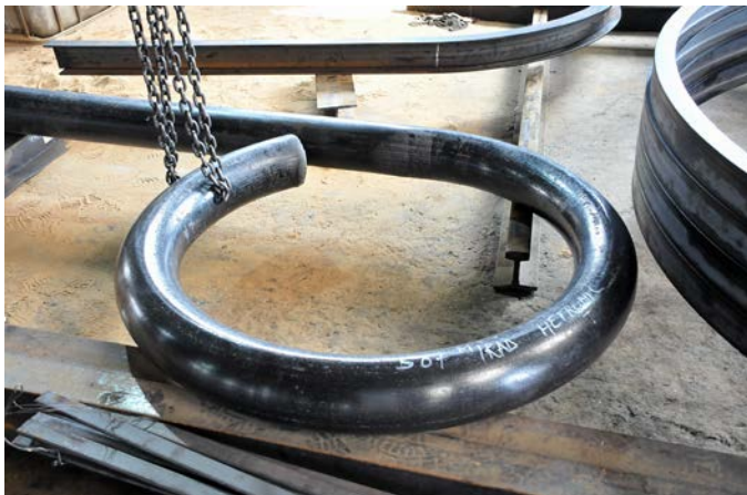
Topping Rollers can bend most sections, in mild steel, stainless steel, aluminium as well as speciality steels. These include angle iron, flat bar, channels, beams, pipes, columns and rails
