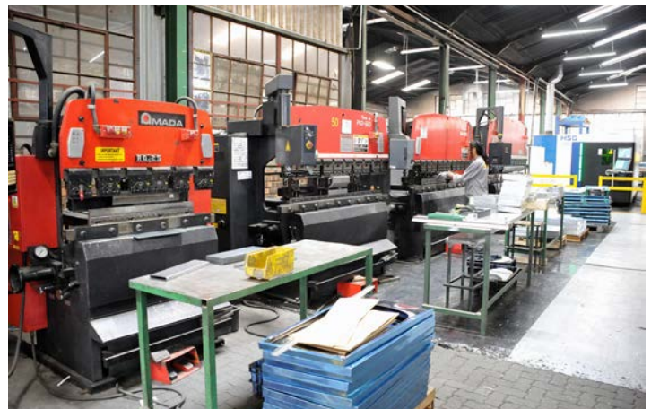
In addition to Pabar's CNC milling and lathe capabilities, it makes use of Amada bending machines and an HSG 12kW G3015X fiber laser cutter with a bed size of 3m by 1.5m. Pabar has a further HSG fiber laser on order
