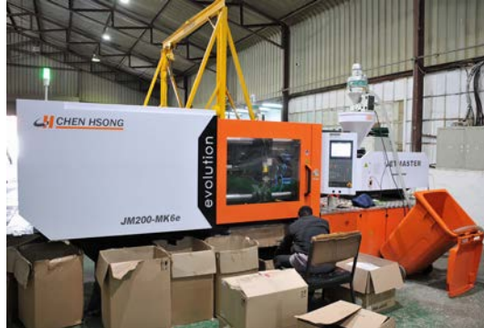
TruSeal have also invested in a Chen Hsong JM200-MK6e moulding machine to manufacture a variety of its plastic seals
