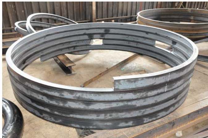
Topping Rollers' capacity is up to 219mm round tube, 300mm by 100mm channel and 305mm by 102mm beam. They are also capable of rolling up to 250mm by 30mm thick flat bars as spirals
