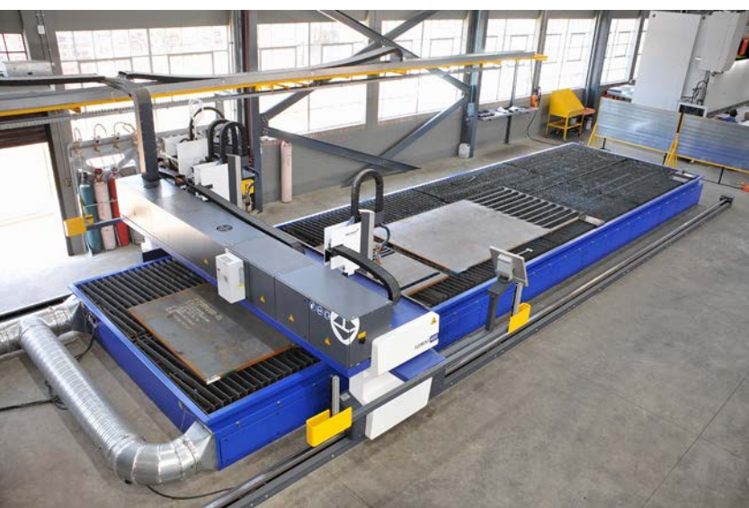
JP Engineering have introduced a new process – plasma and profile cutting – into the processes that they offer with an investment in a Messer Element 400 equipped with a Skew Rotator Delta that is capable of making bevel cuts within an angular range from +45° to -45
