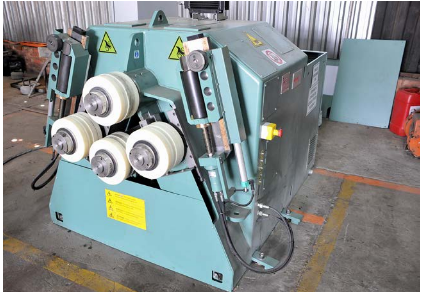
The newest addition to Topring Rollers' shop floor is a Roundo Model 4R3S four roll section rolling machine, which has been supplied by Talmac Machine Tools. Roundo is originally a Swedish company but now is within the Faccin Group. The Roundo Model 4R3S series delivers exceptional performance and outstanding results for small and medium profiles. The four roll machine is a fully CNC programmable section roller
